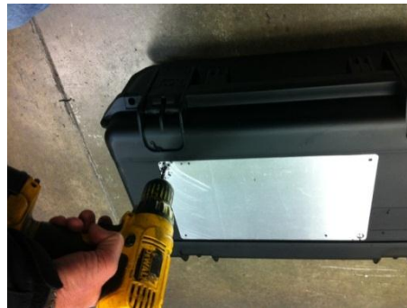
Insert a screw into each hole as you drill them to hold alignment
