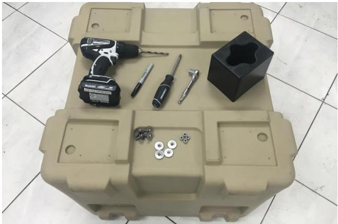
Tools required include a marker, 1/4" drill, Philips screwdriver, 7/16" socket
