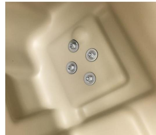
Install sealing washer and then nylon lock nut from the inside and tighten hardware. Note that the washer will form around the one location with the bump.
