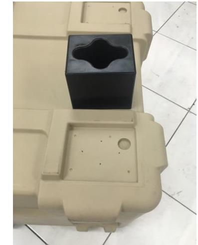
Place riser foot in caster pocket on bottom of case and mark hole locations
