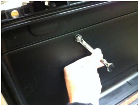
Tighten the screws and nuts using the screwdriver and wrench until the domed washer becomes flat
